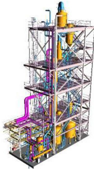
Heat integration (feed/product interchangers) and high efficiency distillation tower packing (to minimize the amount of reflux) are used to reduce the energy requirements of the system.
