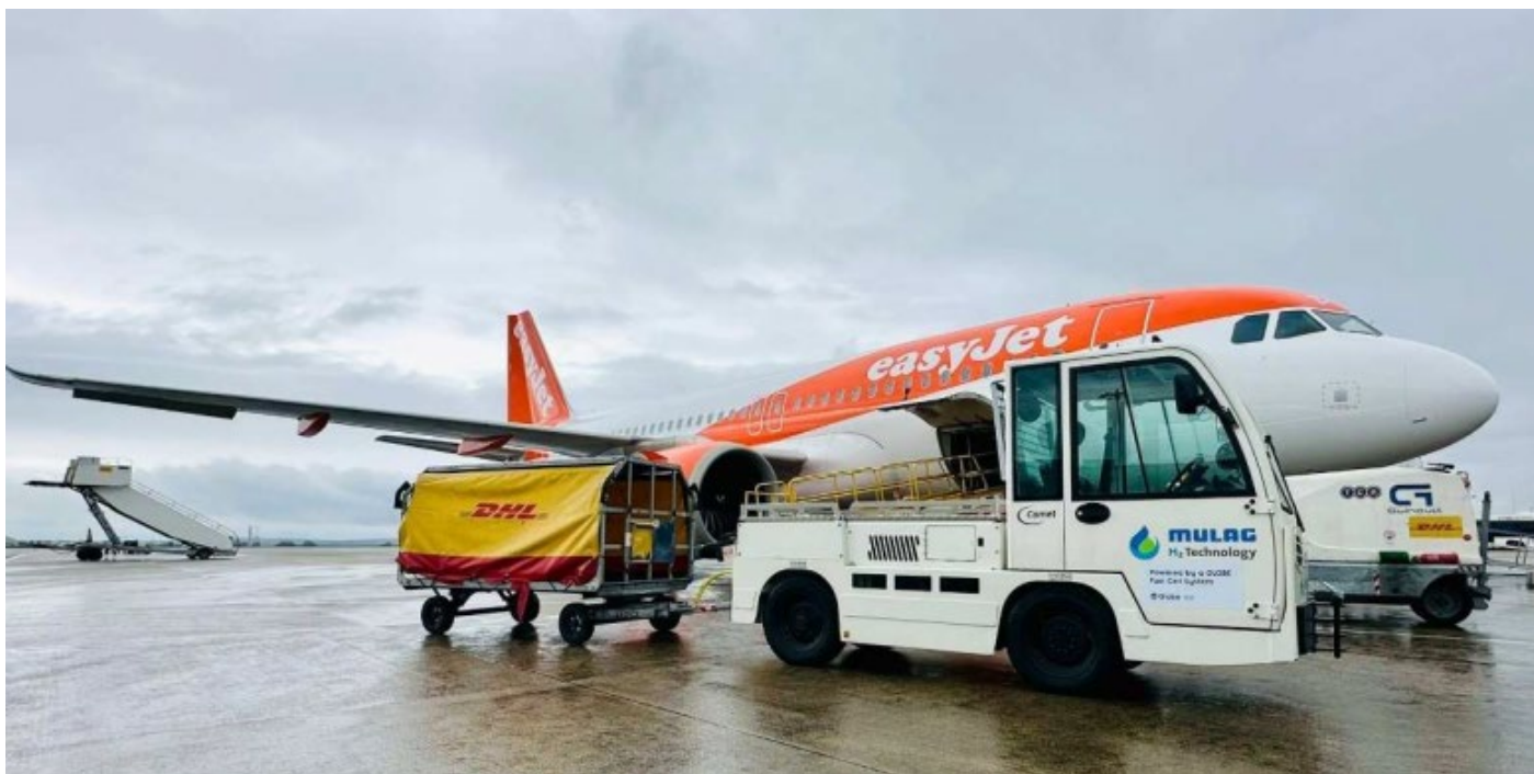
Figure 22: HBT Towing Baggage Trailer at Bristol Airport During Aircraft Turnaround
