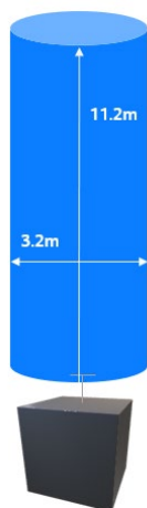
Figure 13: Refueller ATEX Zones from Vent Line
