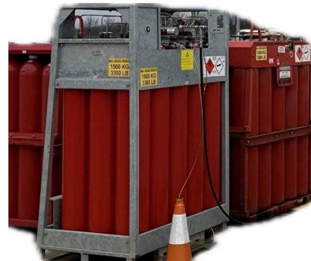
Figure 9: Three MCPs each storing 9 – 10kg of Hydrogen
