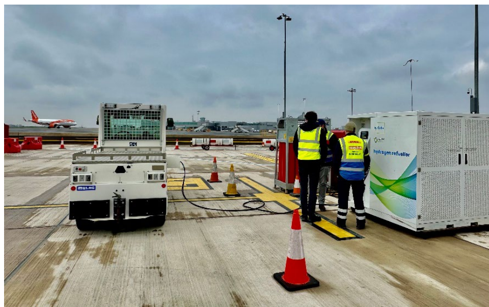
Figure 21: HBT at Bristol Airport During Initial Refuelling
